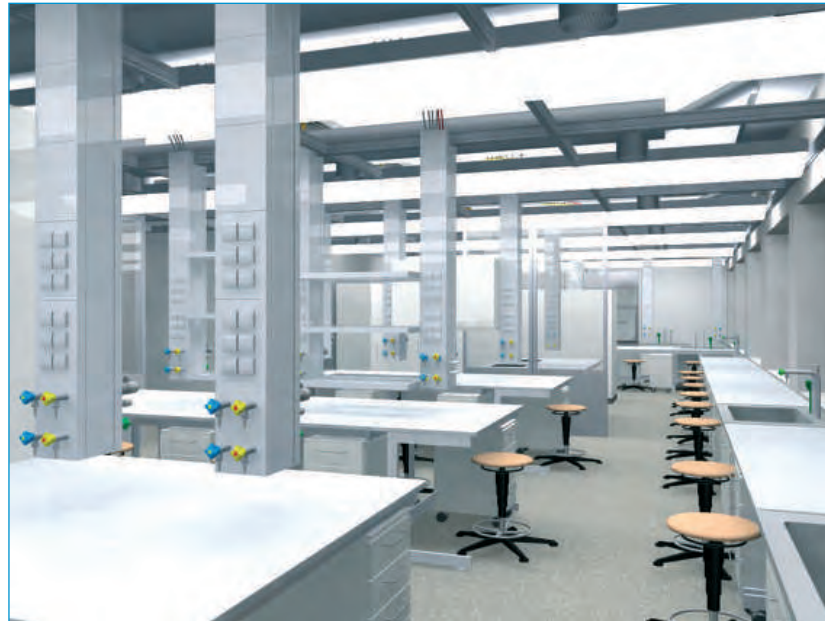
Example for room supply through a service ceiling ■
