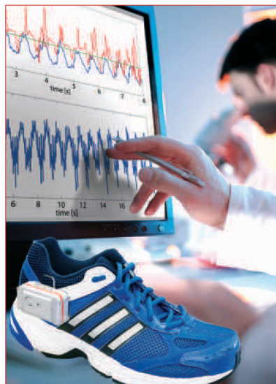
The shoe, which is fitted with a sensor, records the patient's gait. Photo: ASTRUM IT GmbH ■
