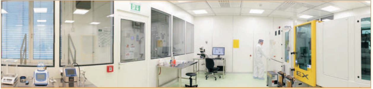
Cleanroom with injection molding machine (collaboration with Gerresheimer AG) ■
