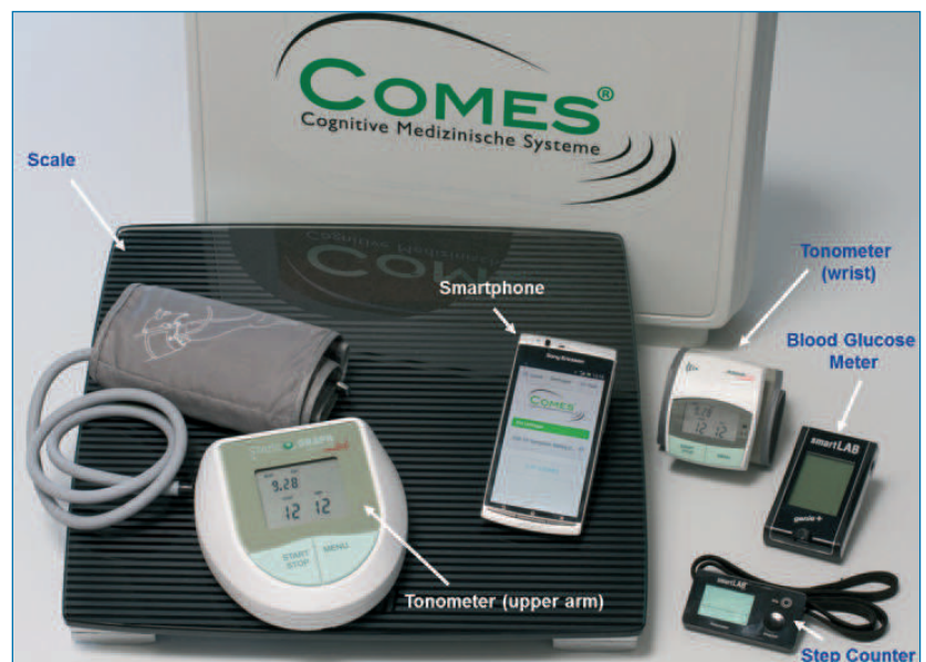
Fig. 1: Telemedical assistance system COMES® developed by the Heinz Nixdorf Chair for Medical Electronics. ■
