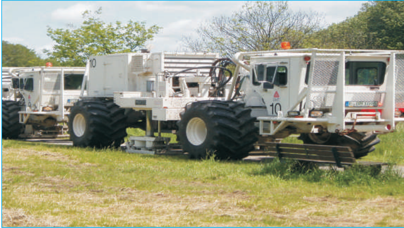
Exploration: special seismic trucks (vibrators) send seismic waves into the subsurface...
