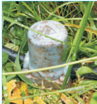
... which are received by a series of small seismographs ("geophones") ...
