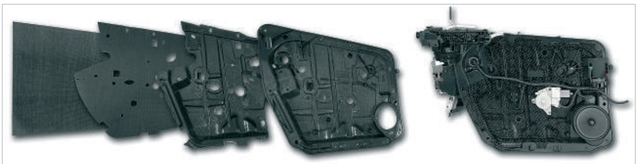
Affordable lightweight design for high-volume manufacturing: the heated mat of glass fabric reinforced polypropylene (thermoplastic composite) is thermoformed into shape in the injection-molding machine while the functional elements of glass fiber reinforced polypropylene are injection-molded ■
