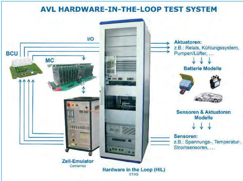
Abb. 2: AVL Hardware in the Loop Test Zyklus ■
