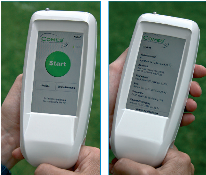
Fig. 2: All-in-one medical device. Left: To collect the relevant vital data, the patient simply slips a finger into the measurement sleeve in the lower part of the device and presses the "Start" button. Right: After a short while the data appear on the display and, if the patient so wishes, may be transmitted to the COMES® telemedical platform via mobile radio ■
