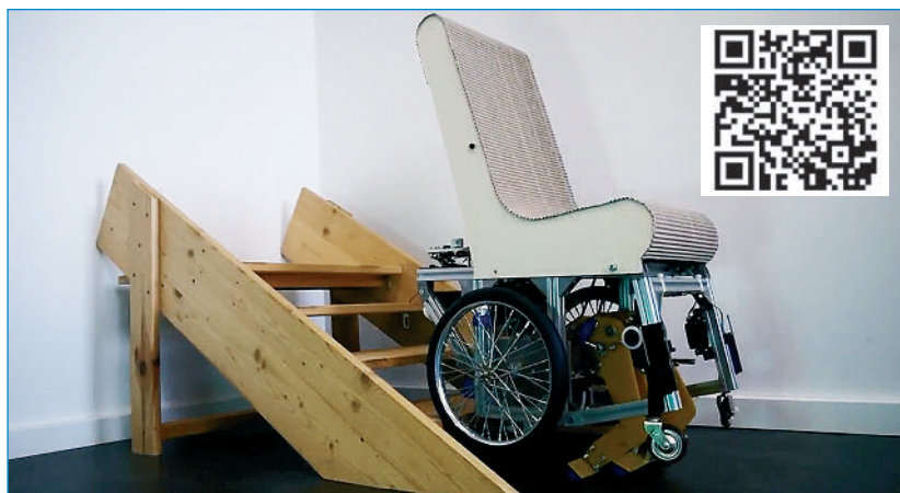
Fig 6: AssistMobil in stair-climbing mode: The two legs (yellow) push the wheelchair from step to step. Scan the QR code (right) to watch a video of a model of the stair-climbing wheelchair in action ■
