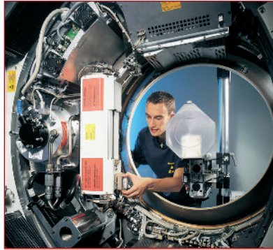
Siemens AG, x-ray tube unit for computer tomography and angiography. Each unit is tested in a Siemens computer tomograph before it leaves the technology centre ■
