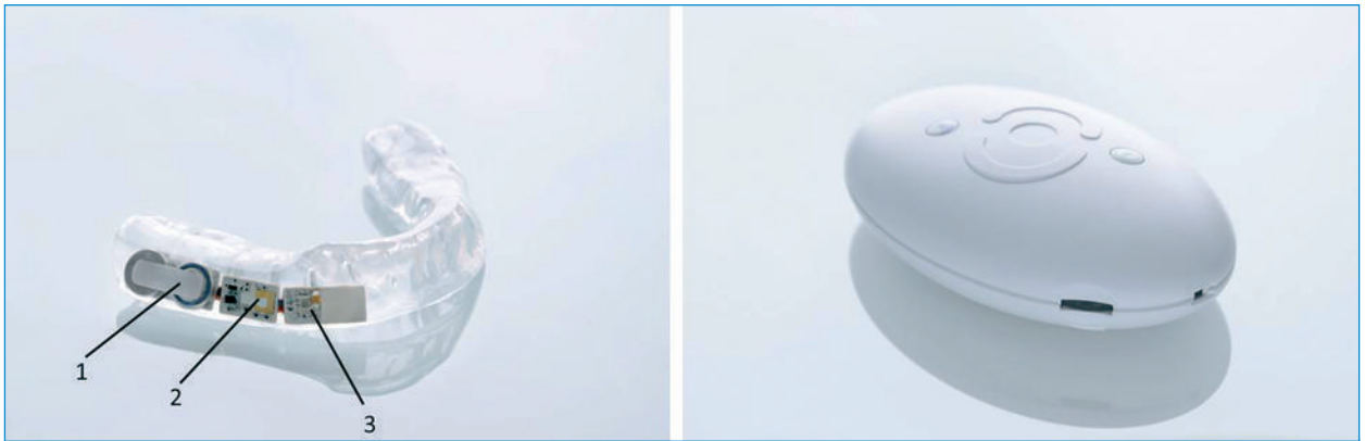
Fig. 4: Left: Intelligent tooth splint with battery (1), sensor unit (2) and antenna (3). Right: Receiver for acquiring data and relaying biofeedback (vibration or acoustic signals) ■
