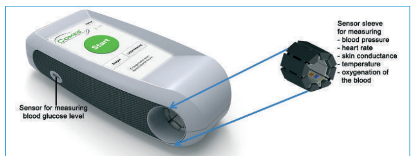
Fig. 1: All-in-One medical device with integrated sensor sleeve (right) ■
