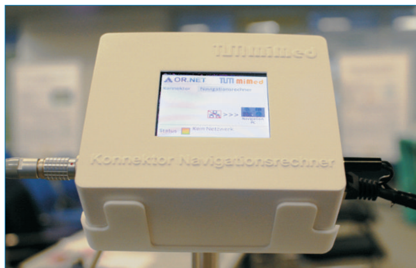
Fig. 2: Connector for the navigation computer. A display shows status information of the device and the network ■
