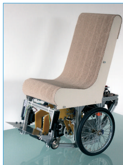
Fig. 5: Model of the “AssistMobil” system. On even ground, the bionic wheelchair is balanced on two large wheels, with the additional legs needed for climbing the stairs (yellow) folded back into the chassis ■
