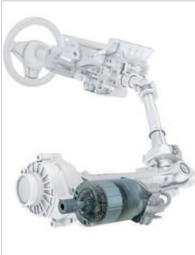
Rack drive for electric steering – as used in the Audi A7 ■
