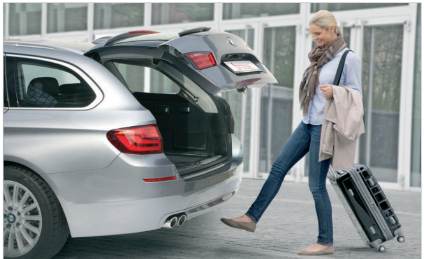
Systems for hands-free opening and closing of liftgates such as Brose's "Hands-Free Access" already demonstrate how sensor technology and mechatronic comfort features can work in unison ■
