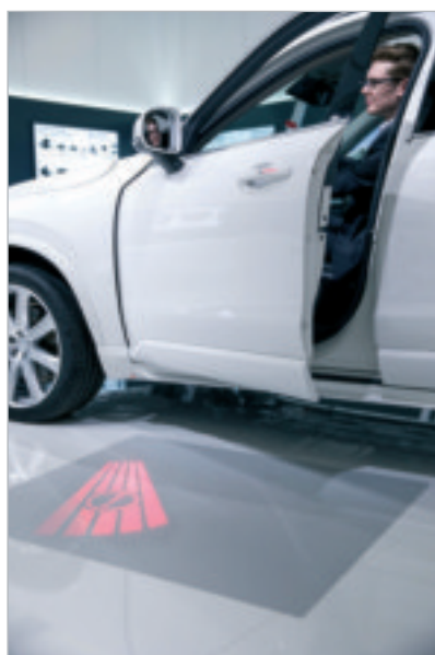
Brose's power side door drive makes vehicle access more comfortable and convenient than ever before. Reliable collision protection is essential if doors open automatically. ■
