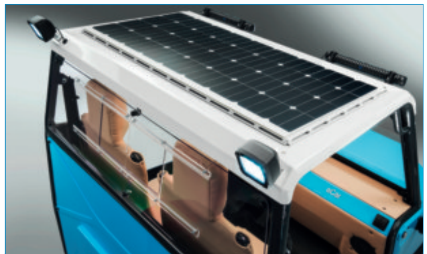
Solar modules are installed on the roof of the vehicle. Credit: Florian Lehmann / TUM ■
