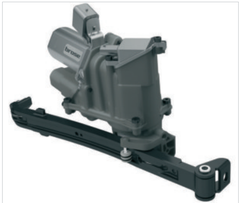
The compact side door drive by Brose can adapt to different customer and vehicle requirements. Series production starts in 2020. ■
