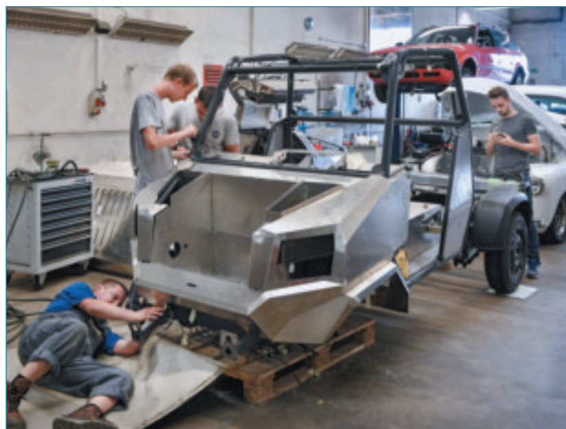
aCar, assembly of the prototype at R & R Fahrzeugtechnik. Photo: Andreas Heddergott / TUM ■
