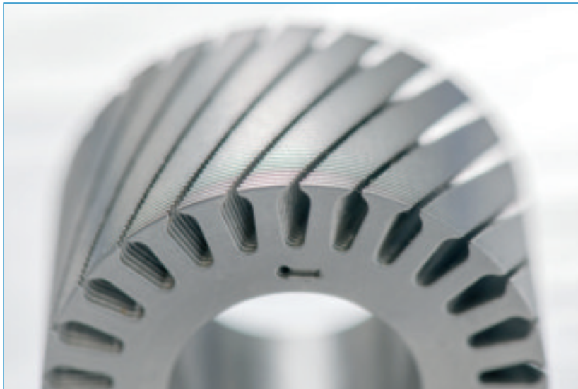
Individual electric sheets are assembled into a compact package. The picture shows a rotor laminated core. (Photo: Andreas Heddergott / TUM) ■
