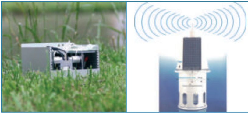
Fig. 4: Water monitoring with the help of biohybrid sensor chips: in a device on the bank of a river (left) and in a buoy for use in a lake (right). ■
