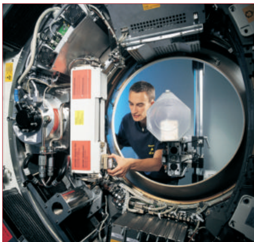
Siemens AG, x-ray tube unit for computer tomography and angiography. Each unit is tested in a Siemens computer tomograph before it leaves the technology centre ■
