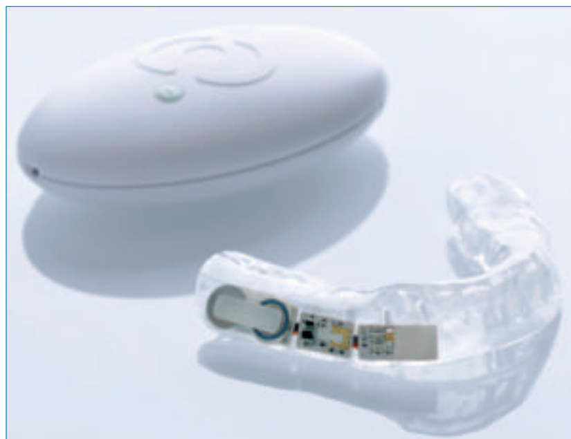
Fig 7: Intelligent dental splint SensoBite with sensor and electronics (bottom) and receiver and vibration unit (top). [11] [12] ■
