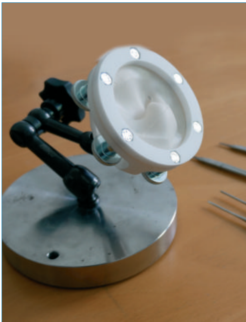
Fig 3: A tangible, patient-specific heart valve replica is ready for the surgeon to inspect and plan a heart valve repair ■
