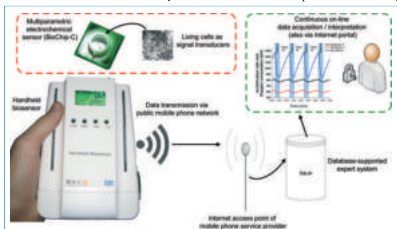
Fig. 3: Functional diagram of the mobile biosensor system microLa ( \mu La) to use with cellristors, e.g. for food control or toxicity tests. ■
