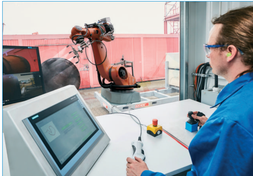
BUCHEN's automated industrial cleaner is controlled with a joystick – by an operator sitting in the control centre (container) well away from the danger zone ■
