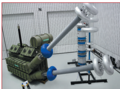
Following a successful final inspection at the Siemens transformer plant in Nuremberg, the world’s first 800-kilovolt ultra-high-voltage power converter transformer is ready for delivery. The transformer will be used in the Yunnan-Guangdong high-voltage DC transmission system in China, currently one of the two HVDC systems with the highest rated capacity in the world. (Siemens press photo) ■
