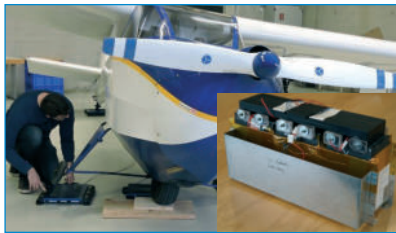
Fig. 2: Battery module developed in the E-Falke project at the Technische Hochschule Ingolstadt ■
