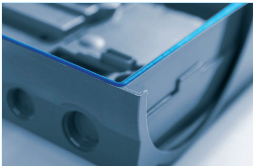
Not only the specific design of the PUR foam seals, for example in terms of density and load-bearing capacity, but also the height and the required deformability can be adapted to the respective product, in this case an electronic housing. © CeraCon GmbH ■
