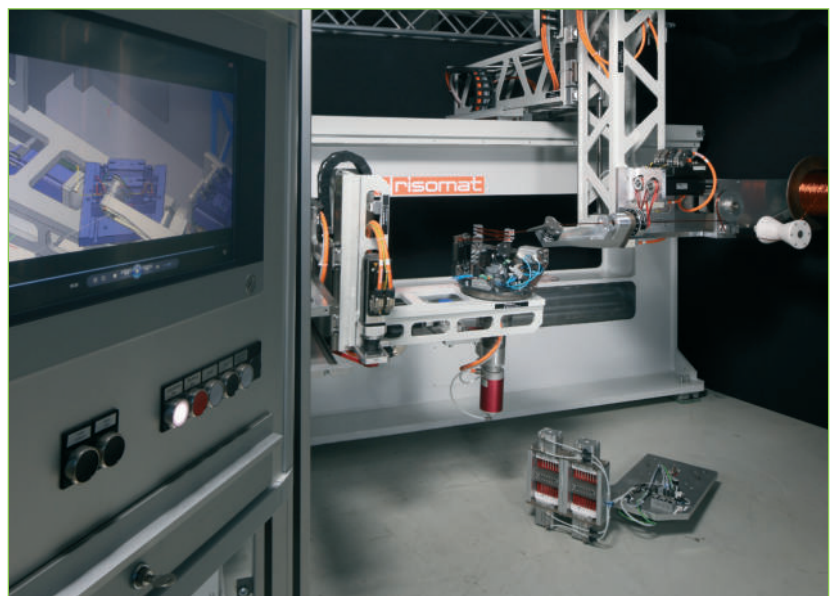
Fig. 4: Innovative universal winding machine for the flexible production of different winding patterns with varying wire geometries ■
