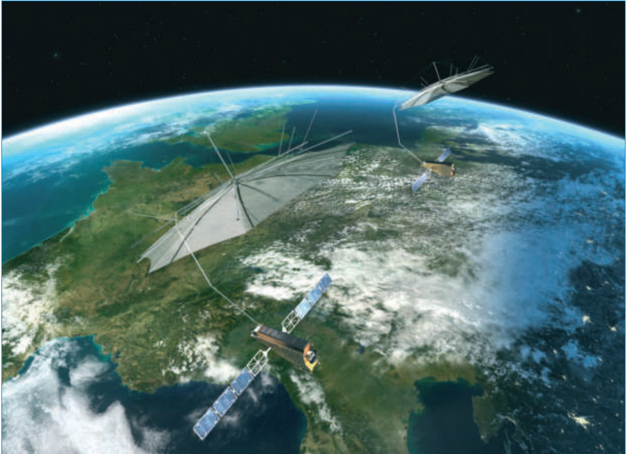
Tandem-L satellites flying in formation; the large, deployable reflectors measure 15 metres in diameter. ■
