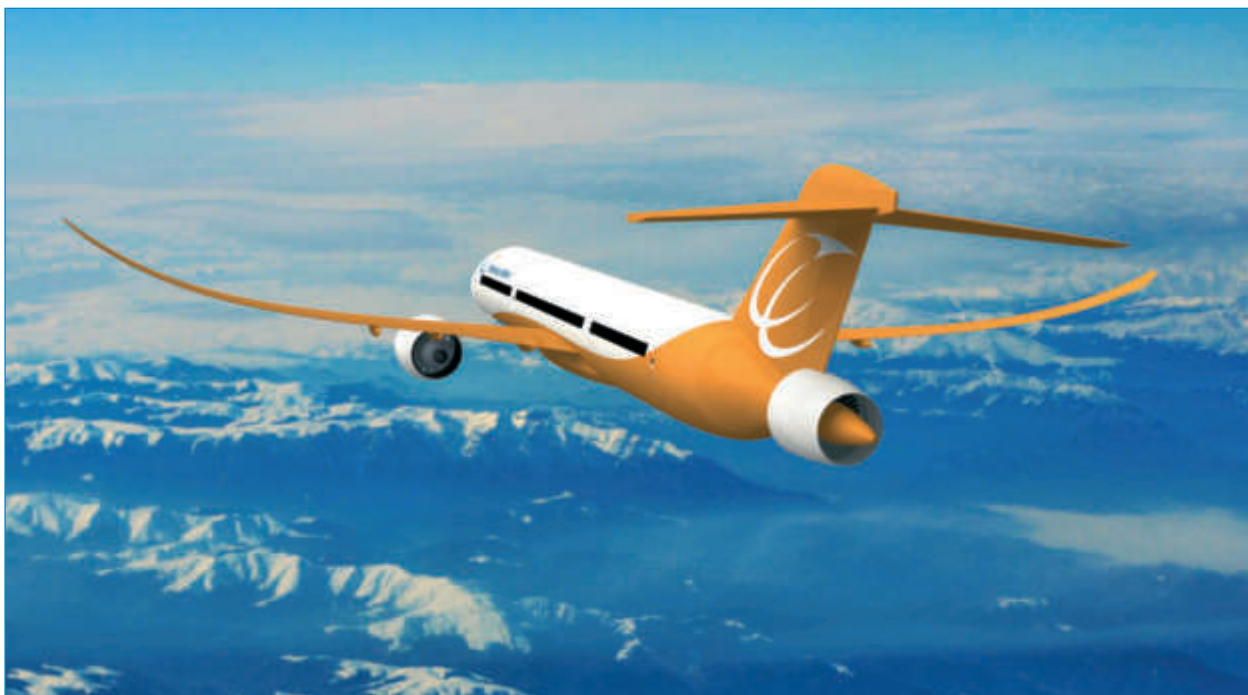
EU-Project „CENTRELINE“ - Synergistic integration of a hybrid electric engine in an aircraft ■
