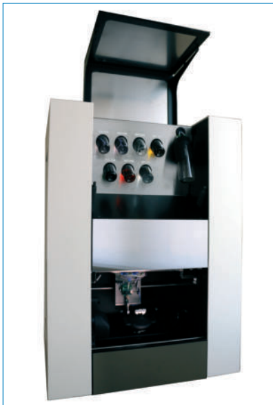
Fig. 3: Left: 5-axis printer for automated coloring of zirconium oxide. Right: Printer nozzle and placed zirconium oxide bridge. (www.softceram.com) ■
