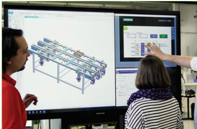
Fig. 3: Kinematic model and virtual control can be combined to verify the system function ■
