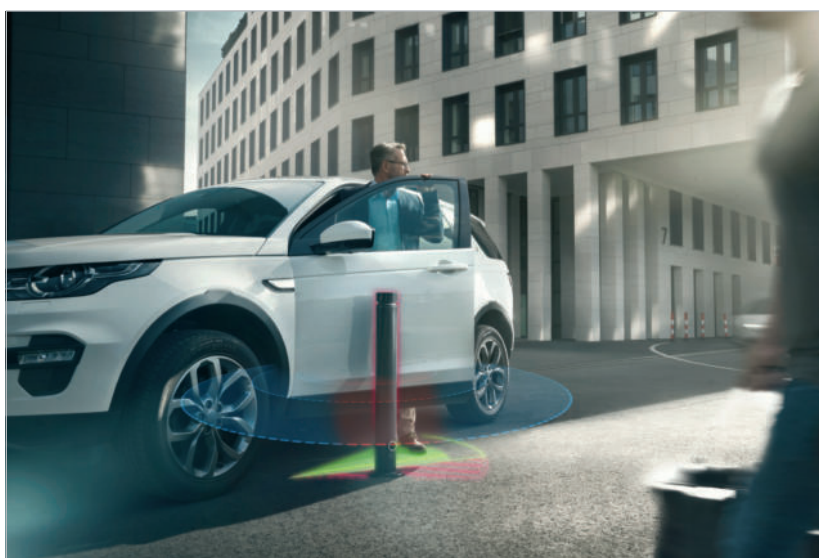
Brose side door drive with radar-based anti-collision protection ■
