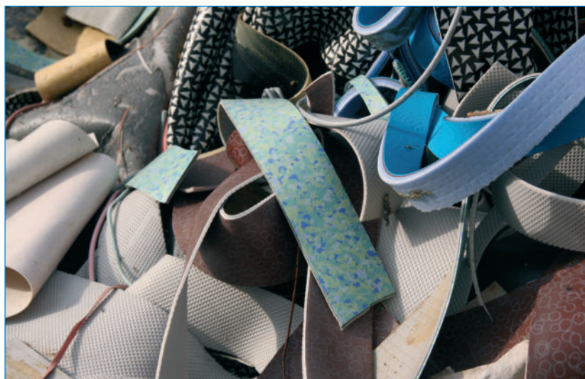
Post-consumer PVC Floor coverings are shredded before entering the CreaSolv® recycling process. Copyright: Arbeitsgemeinschaft PVC Bodenbelag Recycling ■
