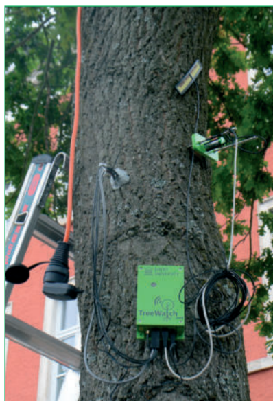
Fig. 2: Development of an internet-enabled "Talking Tree" at high school Wunsiedel. Visible (from left to right) are sensors for measuring water transport (grey), a data logger with transmission unit (green), a dendrometer for measuring tree growth (green, on the trunk top right) and the transmitting antenna (top). ■
